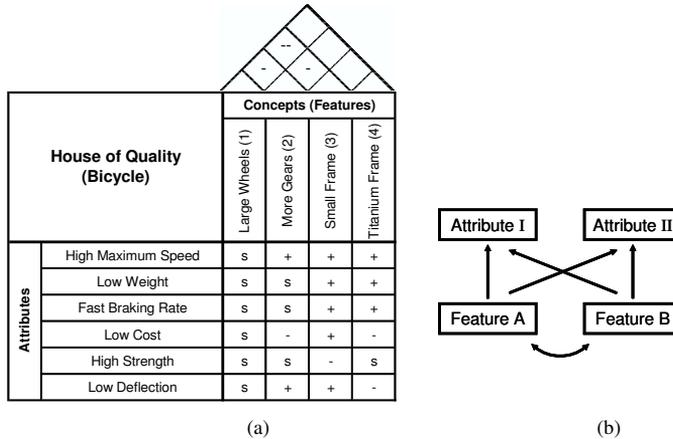
Figure 4. (a) Example of a simplified second HoQ. (b) Evaluation of concepts using second HoQ.
