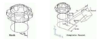
**Figure 2.** Complete Faucet with Knob. The driving parameter set {Wo, Ho, Lo,  $\theta$ 1,  $\theta$ 2} And the Knob radius {Rb} is 0.5Wo.
