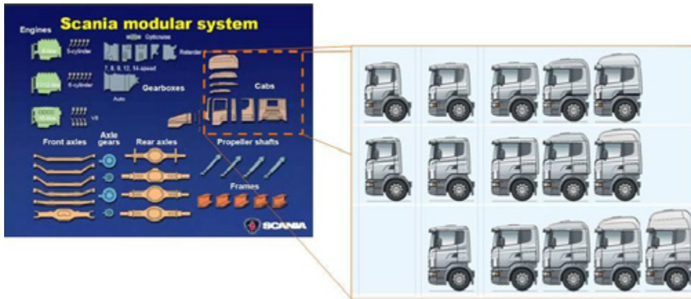
Figure 2: Illustration of Scania’s modular system and possible cab variants [19],[22]
