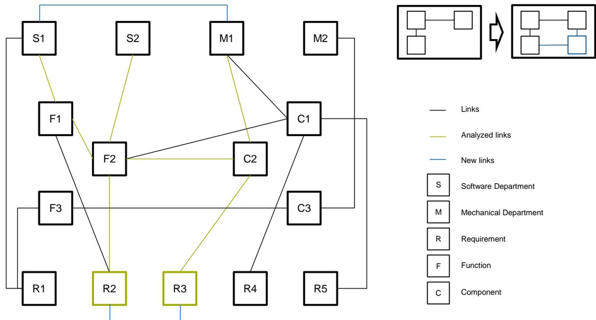
Figure 2. Identification of lacking connections using higher order links
