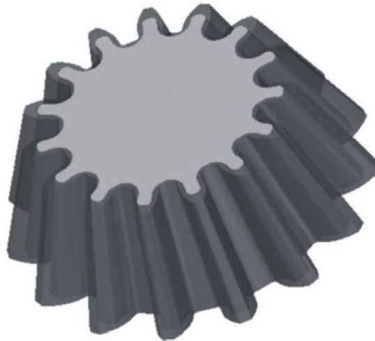
Figure 5. Bevel Gear; inner part aluminium, outer part steel
