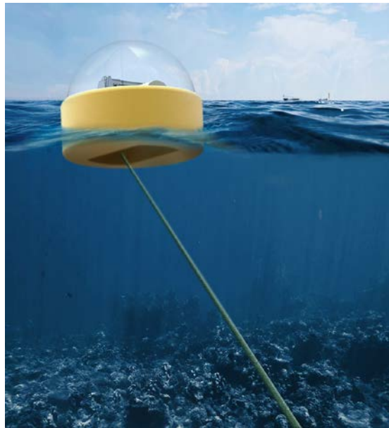
Figure 1 Illustration of a point absorber with a winch-based PTO where the winch is integrated in the buoy (Agge, 2016)
